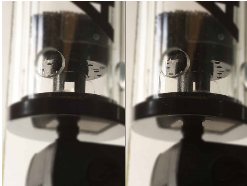
Pict. 2: Regulating the flow is done through adjusting the gap inside the reactor by turning the knob on top of the unit. The pump is connected at the bottom of the unit.
